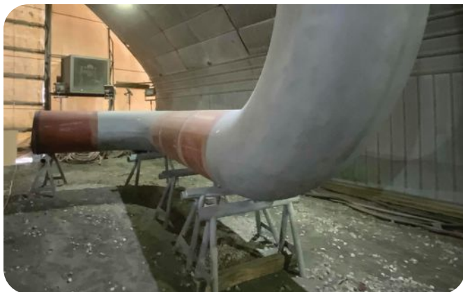
The substrates were blasted with equipment from Marco and Montipower to near-white NACE No. 2/SSPC-SP 10.
